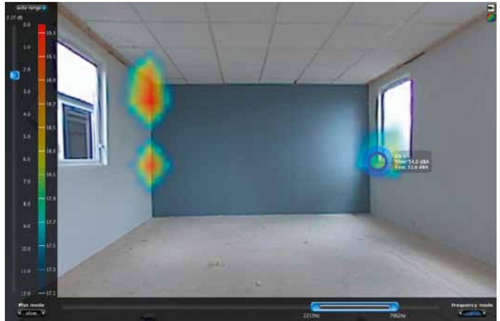
Leakage localization for building acoustics applications
