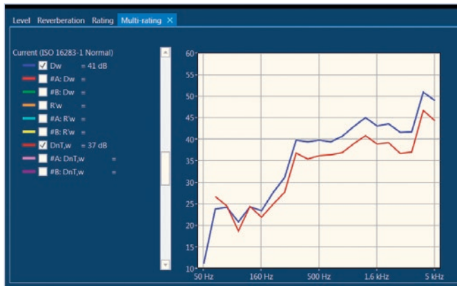
For easy comparisons, the Multi Rating view offer graphically view of multiple measurement results.
